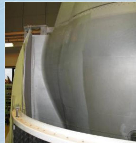
Note – Repair in “Sections” vs One Large Area
