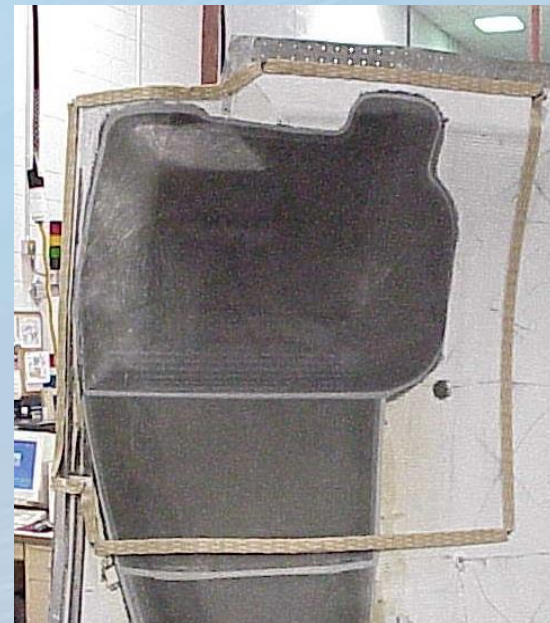
Result – Kit is ready to bag and cure – total time involved in placement --7 mins
