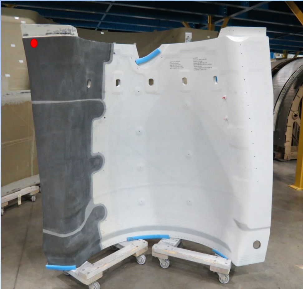
Finished Panel, after heat blanket cure
