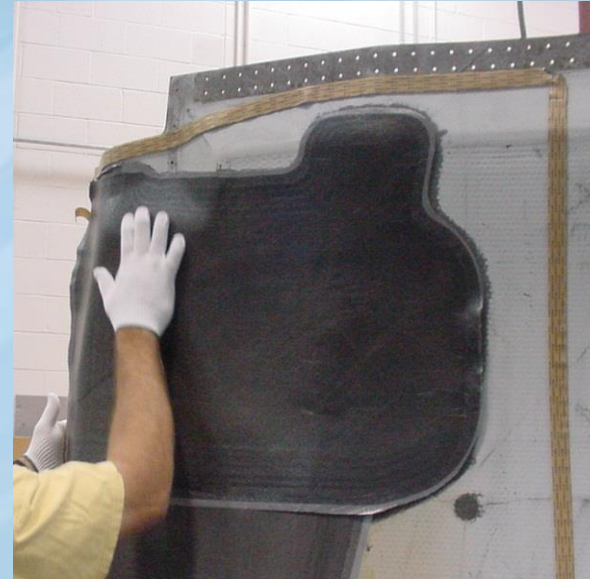
Smoothing kit into sanded recess, tool located and template aligned
