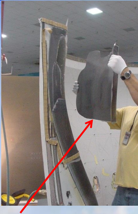
Example of consolidated repair kit, this one was done out of autoclave
