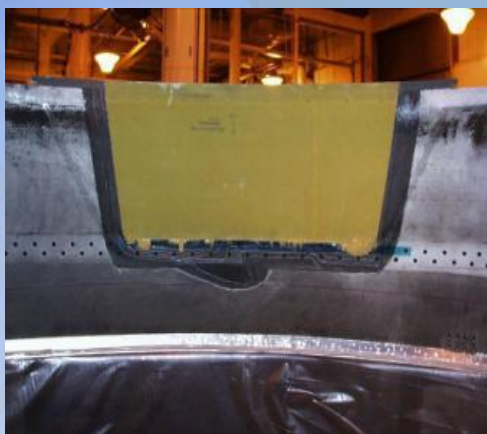
Large Area Trans-Sleeve Repair
