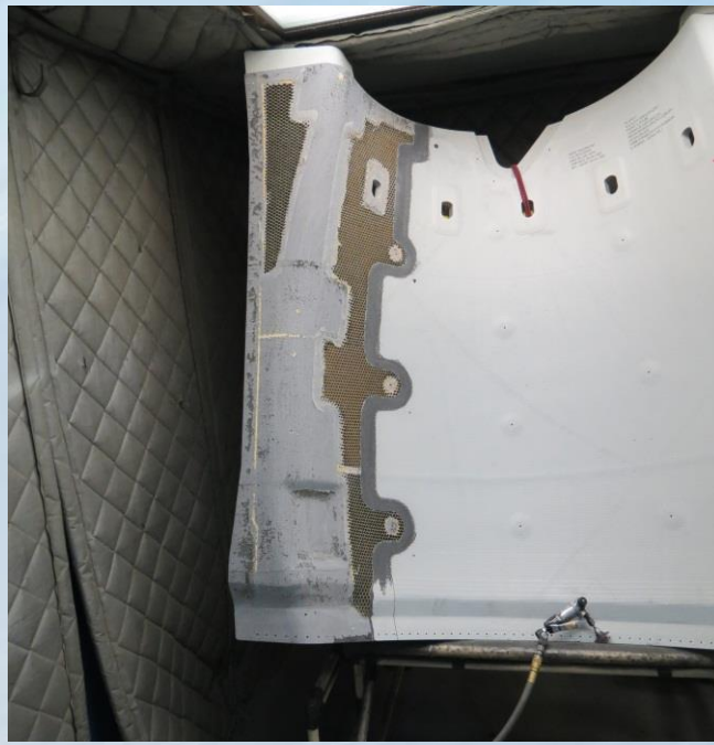
Taper Sanding Removal
