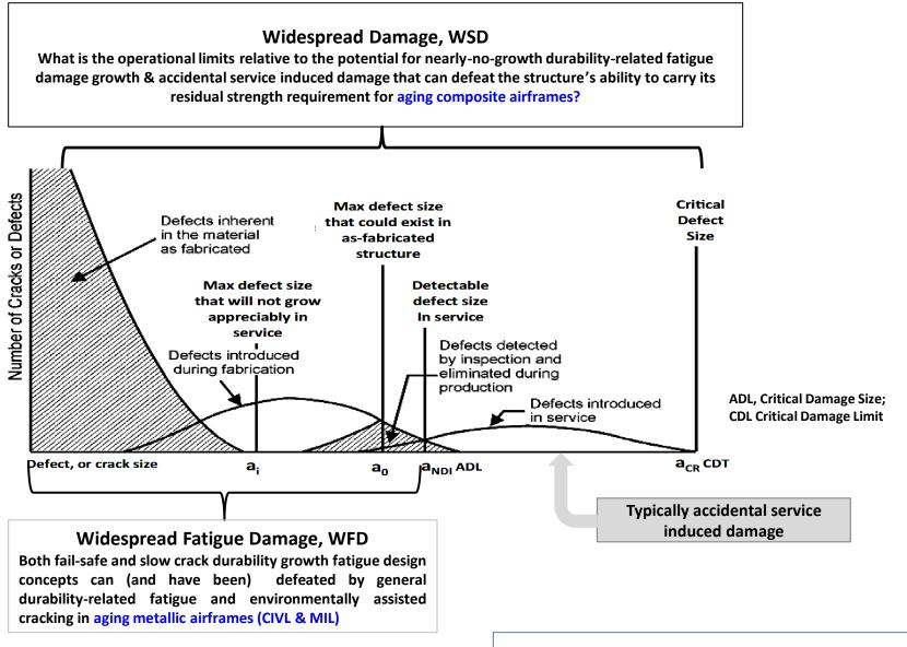
Adapted from E.K. Walker, J.C. Ekvall, and J.E. Rhodes (1979). "Design for Continuing Structural Integrity." Structural Integrity Technology. ASME, NY. Damage Sensitivity of Laminated Composite Systems: Primary is in-plane Loading Notch effects & Secondary Induced-out-of-plane Loading Effects.
