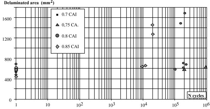
Example : T800/F655-2 material, impacted at 6 joules (around the BVID). Constant amplitude fatigue testing at various ratios of the compressioncompression testing, R = 10 after impact (CAI) strength.
