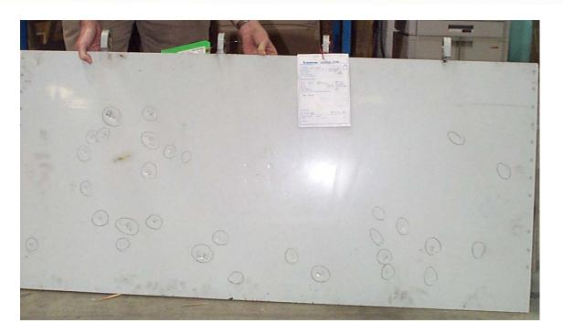
Sandwich construction can be more susceptible to impact and environmental damage but with good design details is minimize
