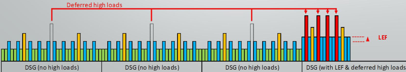
Cycles below composites truncation level (green) are eliminated after 3 DSG
