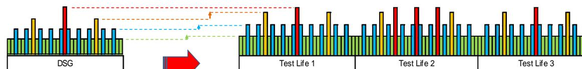
Original Spectrum is multiplied by appropriate LEF with multiple combined load-life factors (example:  $N = 3 < N_F$  for  $LEF_2 = LEF_3 = LEF_4 \neq LEF_1 = 1.0$  with  $N = N_F$ )
