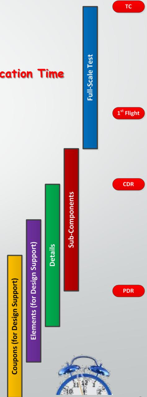
Full-scale test is a significant portion of the overall budget
