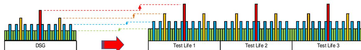
Original Spectrum is multiplied by appropriate LEF with combined load-life factor (example:  $N = 3 < N_F$  for  $LEF_1 = LEF_2 = LEF_3 = LEF_i$ )
