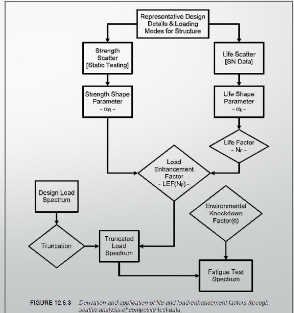
FIGURE 12.6.3 Derivation and application of life and load-enhancement factors through scatter analysis of composite test data.
