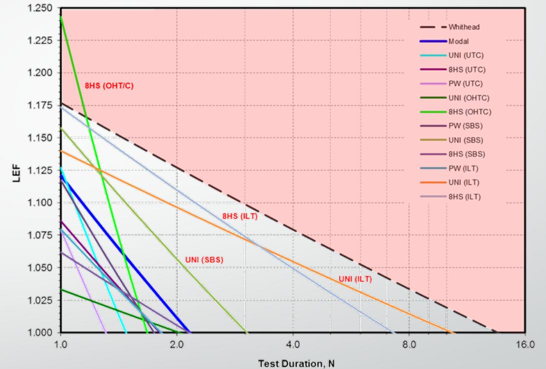
Failure modes with large scatter shall be interrogated at element/sub-component level(s)
