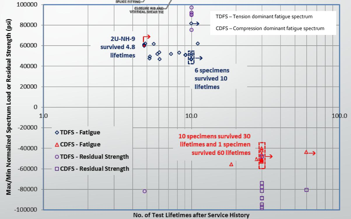
Ref: Seneviratne, W., et al., "Durability and Residual Strength Assessment of F/A-18 A-D Wing-Root Stepped-Lap Joint," 11th AIAA Aviation Technology, Integration, and Operations (ATIO) Conference and the Centennial of Naval Aviation Forum, September 2011.
