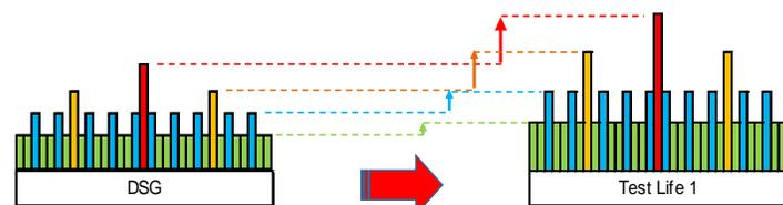
Original Spectrum is multiplied by LEF for N = 1 with Load Factor ( $N = 1$  for  $LEF_1 = LEF_2 = LEF_3 = LEF_4 = LEF_{@N=1}$ )
