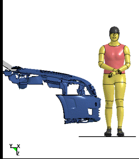
Car to 5th Female Pedestrian Collision (FE Simulation) Time = 0
