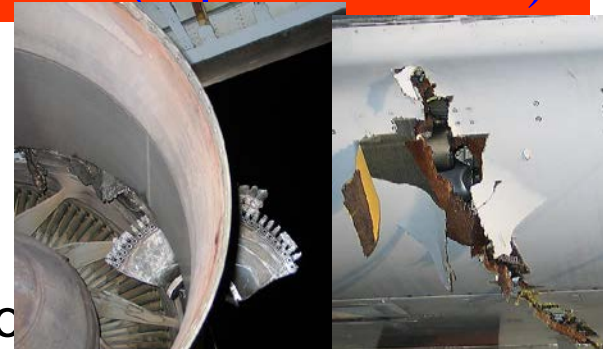
Rotor Disk Cut Through the Aircraft Fuselage Belly and Wing Center Section to Reach Opposite Engine
