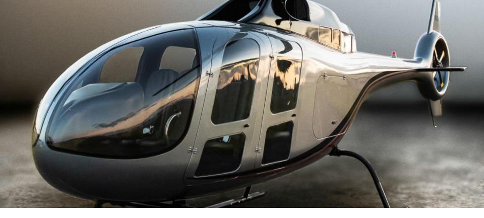
Fully articulated main rotor & ducted fan tail rotor
