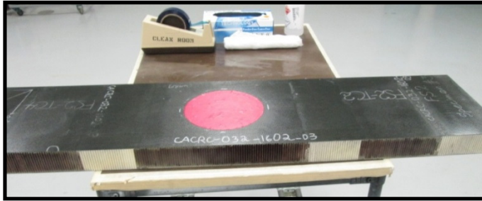
Adhesive application – prepreg repair
