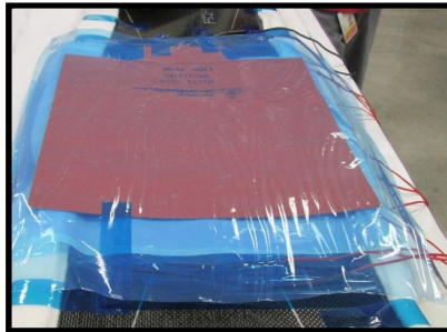
Heat Blanket Application
