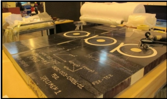
CACRC Repair Element Masking in Preparation for Scarf Sanding
