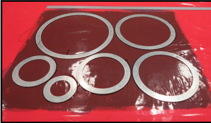
Wet lay-up ply impregnation
