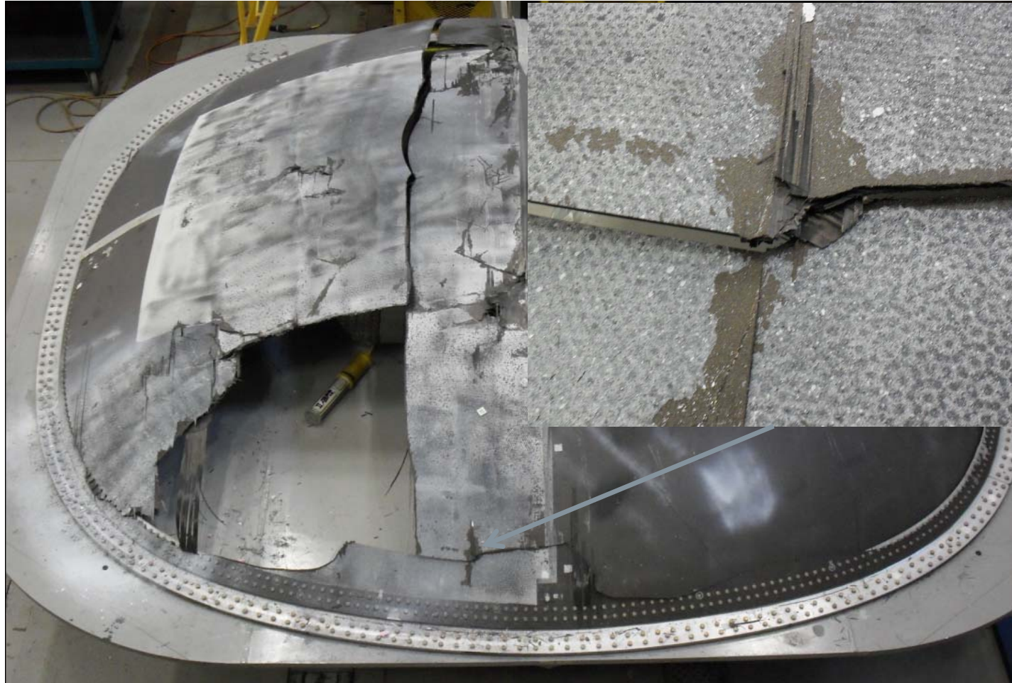
Similar failure mode on un-configured plate
