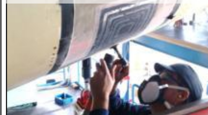
Skin perforation and two stringers disbonded
