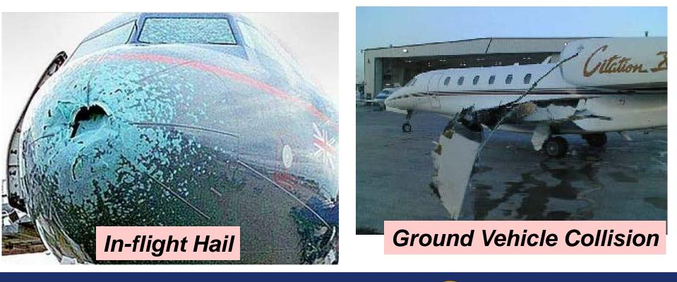
FAA Composite Damage Tolerance & Maintenance resented at 7/19/06 Composite Workshop (July 19-21, 2006) Damage Tolerance & Maintenance
