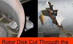
Rotor Disk Cut Through the Aircraft Fuselage Belly and Wing Center Section to Reach Opposite Engine
