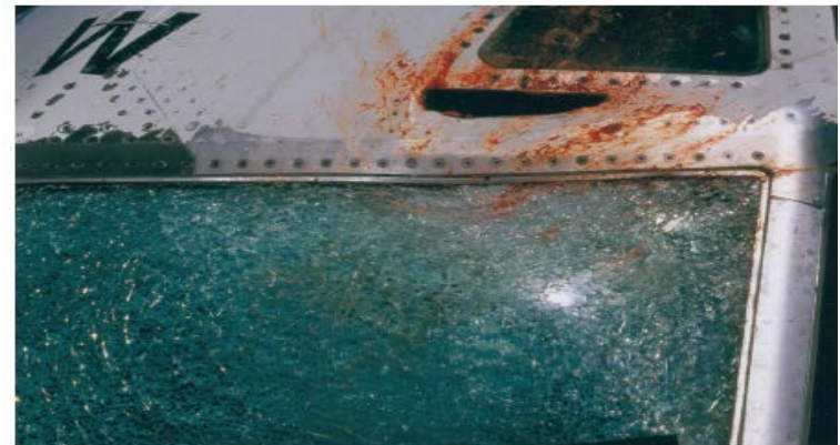
Plate 11 The windshield on this B737 was severely damaged as a result of a collision with a bird at 10,000 ft. ASL and 250 kts. The captain was injured from debris when the bird penetrated the fuselage above the windshield.
