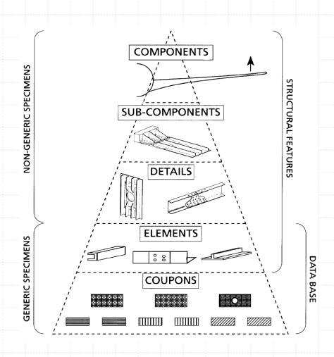
•Data from sources like CMH-17 and NCAMP data at the coupon level, and may not provide all the coupon level data needed to support a specific design.
