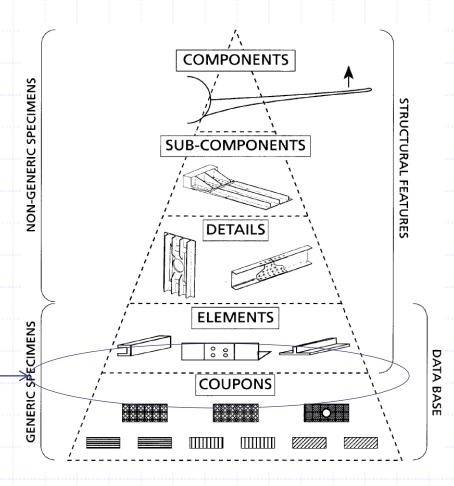
•Final selection of coupons needed to derive design values must take into account values needed by the analytical tools used in the design of actual details and components.
