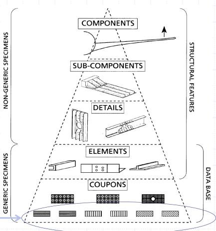
•In order to encompass the variations introduced by both the materials and fabrication processes used, design values must be determined from testing of coupons which sufficient complexity to reflect the sources of variation.
