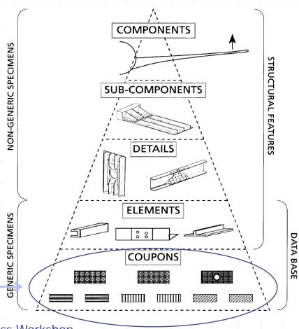
•Testing at the lowest levels are vital for the development and validation of material specifications, but may be of limited use for deriving design values
