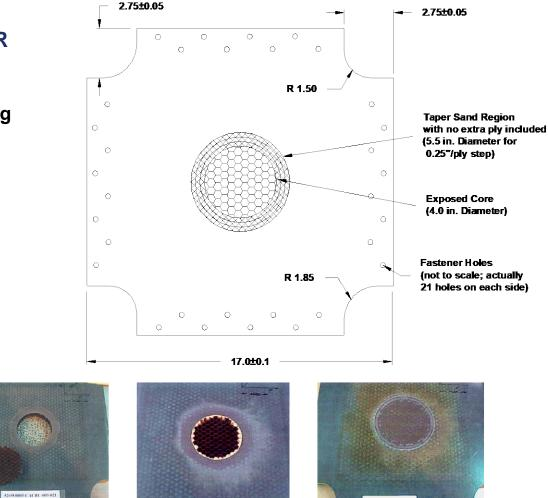
FAA R&D in Composite Sandwich Structures 20 July 2006
