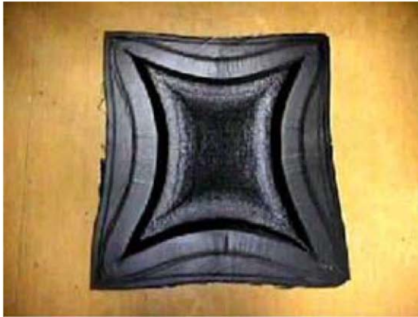
FIGURE 5.4.1(b) Panel exhibiting substantial core crush.
