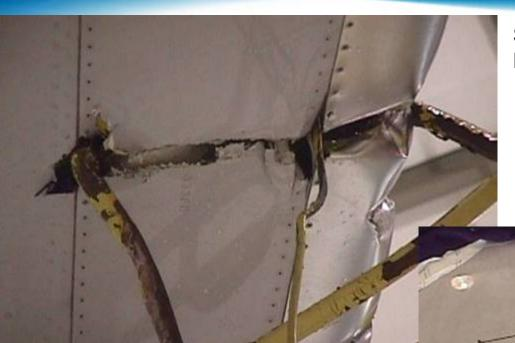
**Skin/Spar Damage—Ground Handling Equipment Impact**
