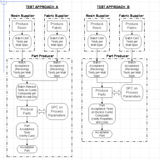
\* Batch testing of combined fiber and resin are completed at the Part Producer for LRM (differs from prepreg materials where it is done at the material supplier)
